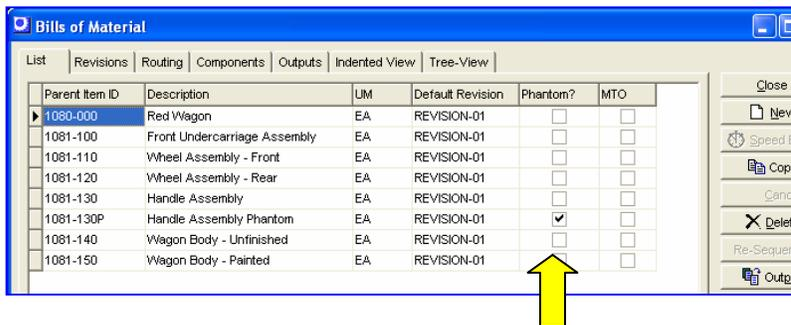
A “phantom” assembly is never stocked and does not have its own routing. When a job is created for a BOM that contains phantom assemblies, each phantom assembly’s components get pulled into that job. If a phantom assembly contains a component that also happens to be a phantom assembly, its components get pulled into the job as well. Thus you can have phantoms within phantoms.
